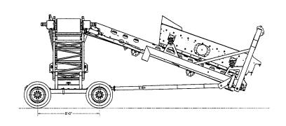
NOTE: CART AND CONVEYOR ASSEMBLY CAN BE ROTATED IN 90 DEG INCREMENTS
